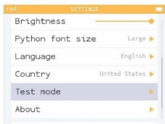
2. Navigate down and press the right arrow or OK to enter Test mode.
